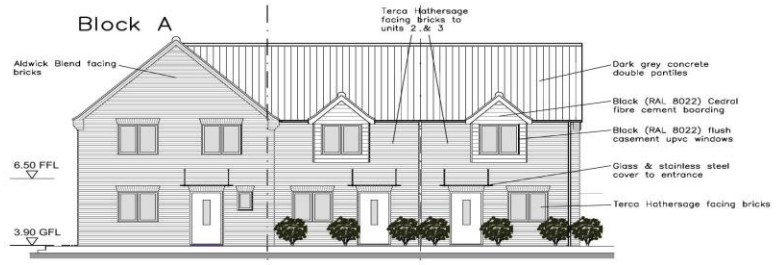
Front East Elevation
